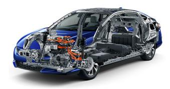
ACE utilizes a network of connected structural elements
