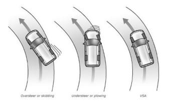
VSA's traction-control function helps maintain stability and allows the vehicle to accelerate even on surfaces with a split coefficient of friction, such as when one wheel is on ice and the other is on dry pavement.
