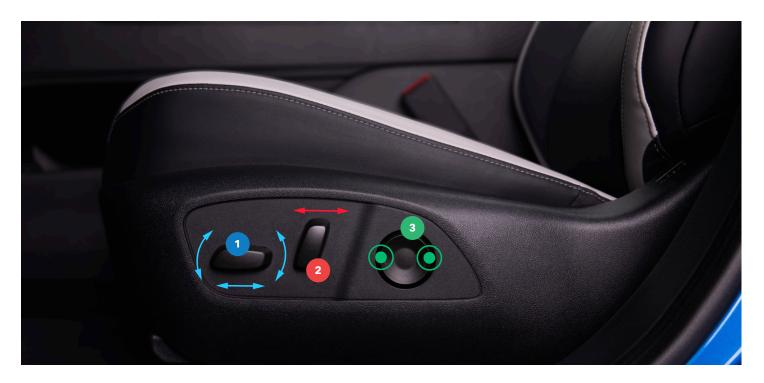
The driver's and front passenger's power seats can be adjusted with the controls on the outboard side of each seat cushion.
