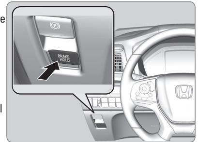
**To deactivate:** To turn off brake hold, press the brake pedal and press the BRAKE HOLD button again.
