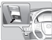
**To deactivate:** To turn off brake hold, press the brake pedal and press the BRAKE HOLD button again.
