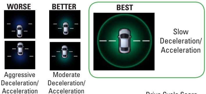
**Drive Cycle Score/Lifetime Points** appear for a few seconds when you set the power mode to VEHICLE OFF. Depending on your driving style, the leaf icon(s) and the gauge increase or decrease to indicate that you have reached a different stage of fuel economy.
