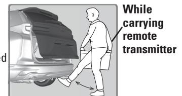
A beep sounds and exterior lights flash **after** the kicking motion has been performed properly as confirmation that the hands-free access has been activated.
