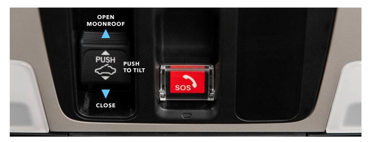
With the power ON, you can open, close or tilt the available moonroof as you desire. To close the moonroof, push the switch forward firmly and release.
