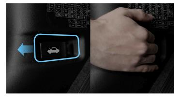
Pull the hood release handle under the driver's side lower corner of the dashboard-the hood will pop up slightly
