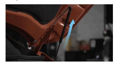
Lift the hood most of the way up; the hydraulic supports will lift it the rest of the way and hold it up
